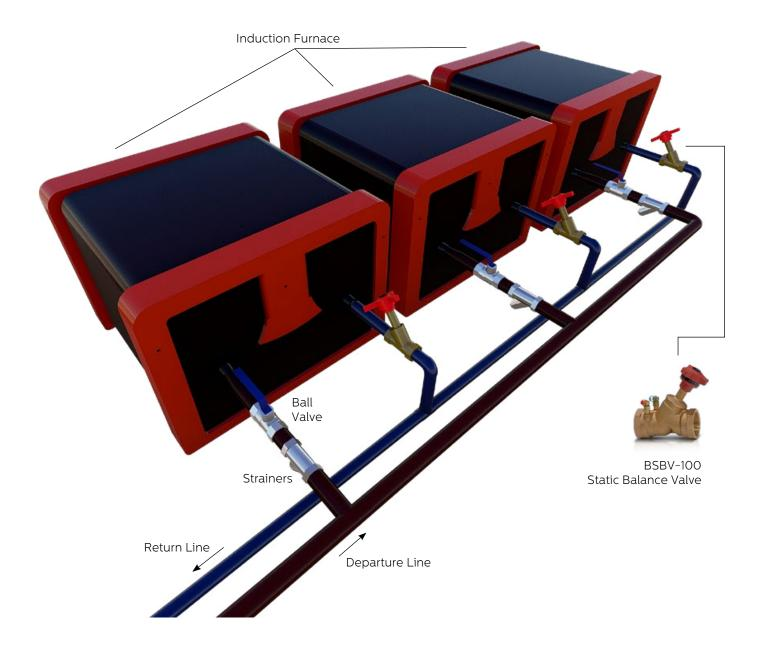
**Note:** It prevents the flow above the required cycle for heat transfer and ensures a more reliable, balanced and healthy operation of the system. It can be adjusted manually by the manuel adjustable throttle disc on it. It is useful to put it on the return line for efficiency.
