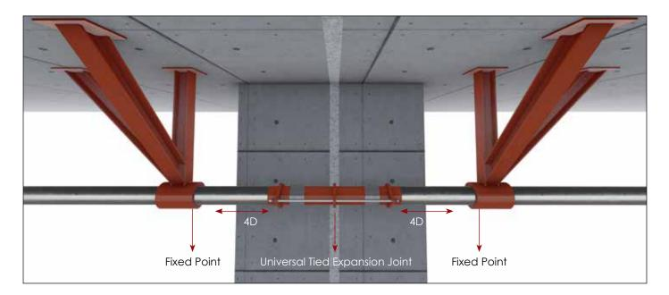
A gap which is equal to the movement amount of the expansion joint should be left between the joint and the construction elements like walls and ceiling. Both ends of the expansion joint should be fixed to each building with the distance of 4D
