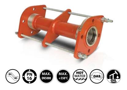
Lateral movement is movement perpendicular to the bellow's longitudinal axis. Thermal movement in pipeline occured in two directions can be absorbed by using Lateral Epansion Joints. Universal tied expansion joints are made up of two bellows connected each other by an intermediate pipe and a system of tie rods able to withstand the thrust resulted of the internal pressure (restrained).
