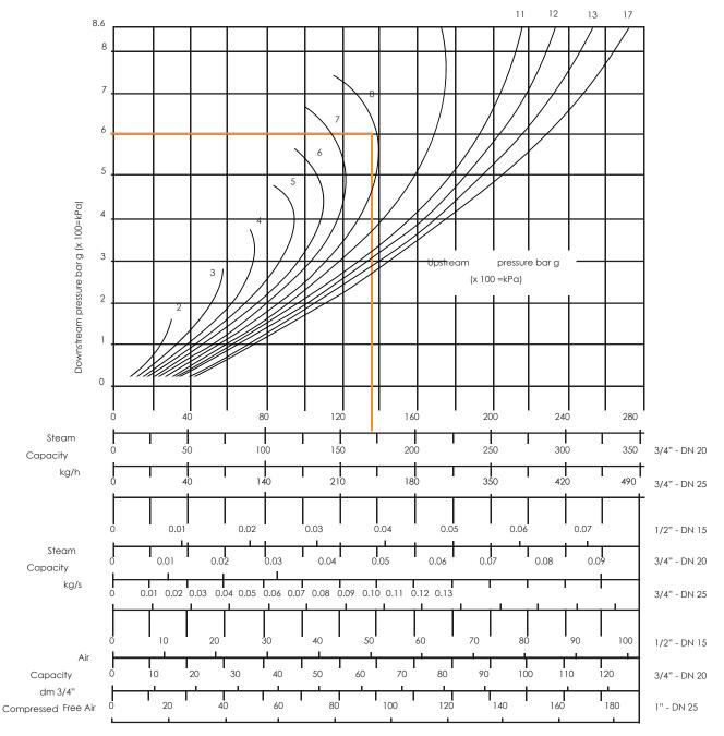
**Example:** required reducing valve to pass 120 kg/h reducing from 8 to 6 bar. From the downstream pressure of 6 bar on the left hand side of the chart to be extended out horizontally until the line. Meets the curve of 8 bar upstream line. Orthographic projection of this point is read as the capacity of the product.
